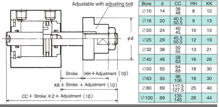
The size shown in the above-mentioned CC cell represented both the value with magnetic and without. The upper value is the size without magnet, and the lower value is the size with magnet.
